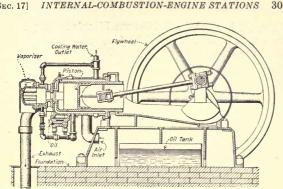
Fig. 282.—Section through a small low-pressure oil engine of the "hot-bulb" or "hot-ball" type.
